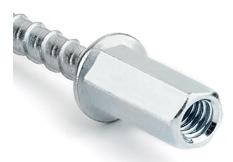
**TFF Head. Female thread with double** M8/M10 thread, for direct, quick and easy fastening of threaded rods in ceilings (concrete and hollow-core slabs). Suitable for suspension of air conditioning ducts, cable trays, pipe systems, etc.
